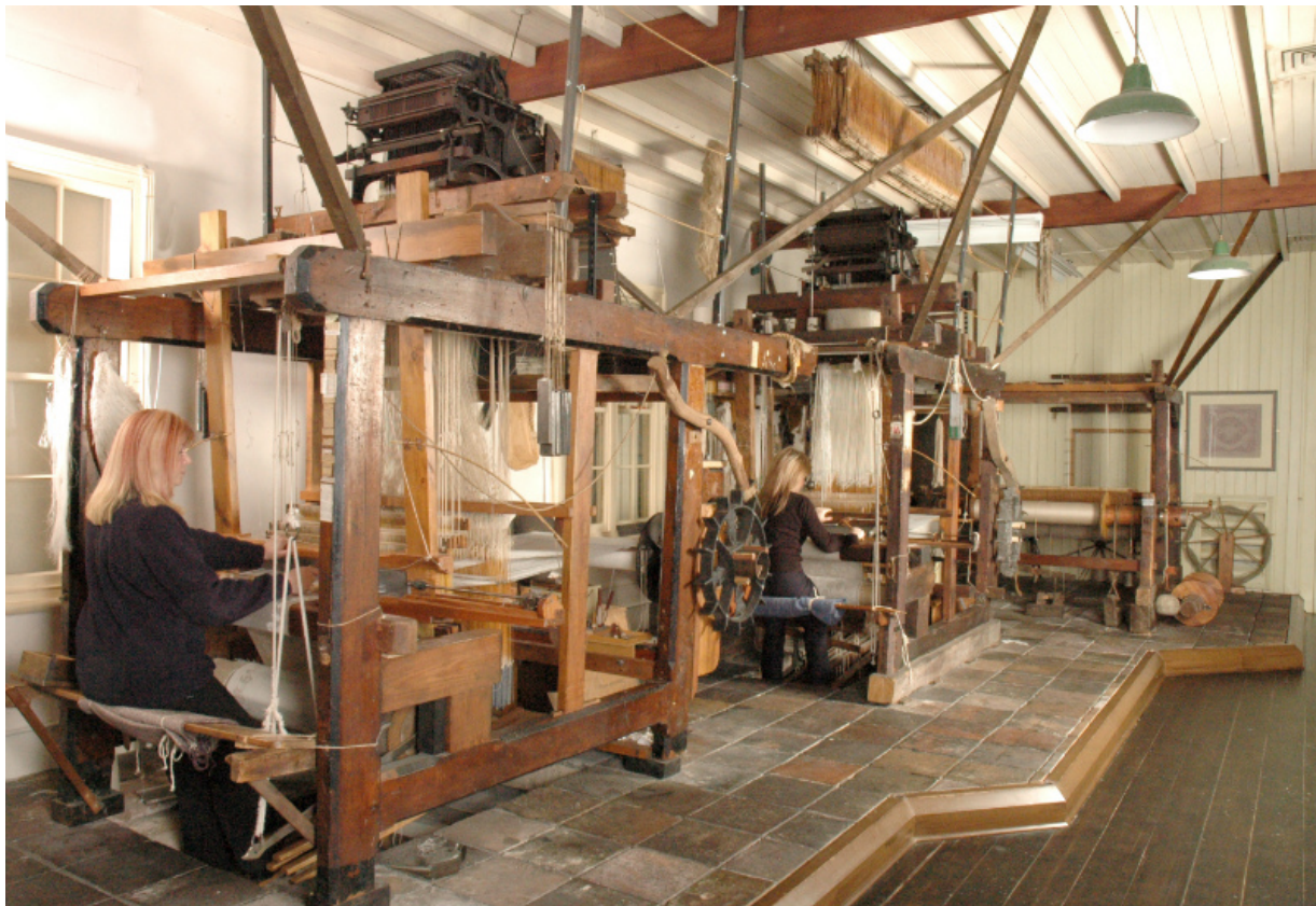
Jacquard Looms in the weaving workshop. Note the mechanism for reading the punched card on top.
